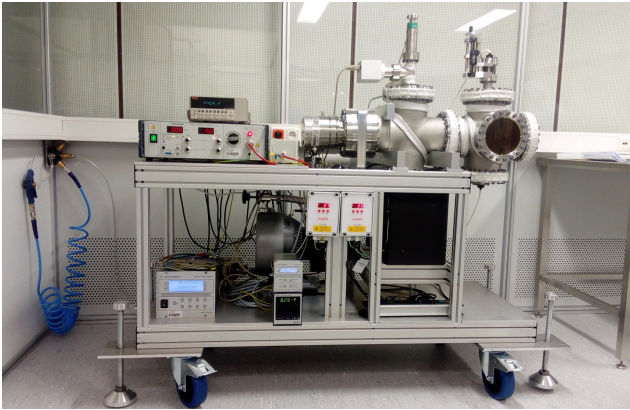
Fig. 1: The test bench for electrostatic deflectors.
